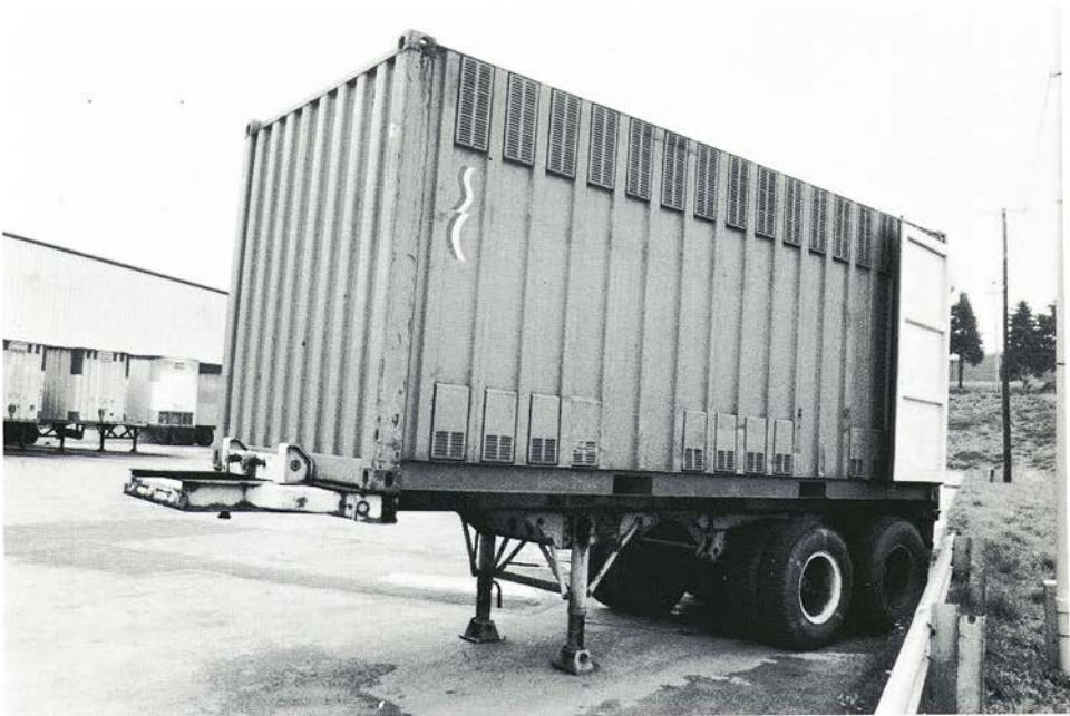
Fig. 3. Driver's side of SCXU 898175-1. Note ventilators along top and bottom side rails.
