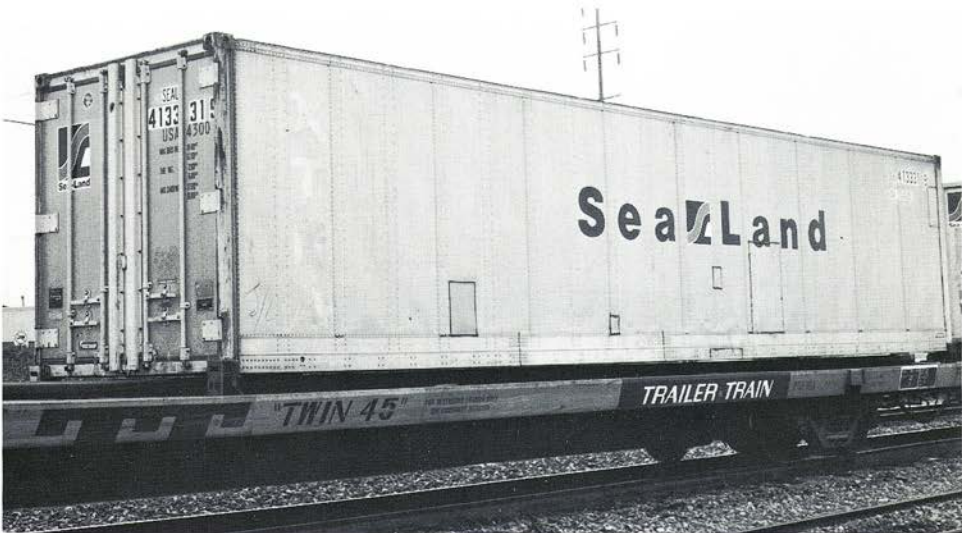
Fig. 2. SEAU 413331. In 1984, Sea-Land Service acquired a number of former XTRA containers like the one shown here. These are 40-foot, non-vented, aluminum containers built by Fruehauf.
