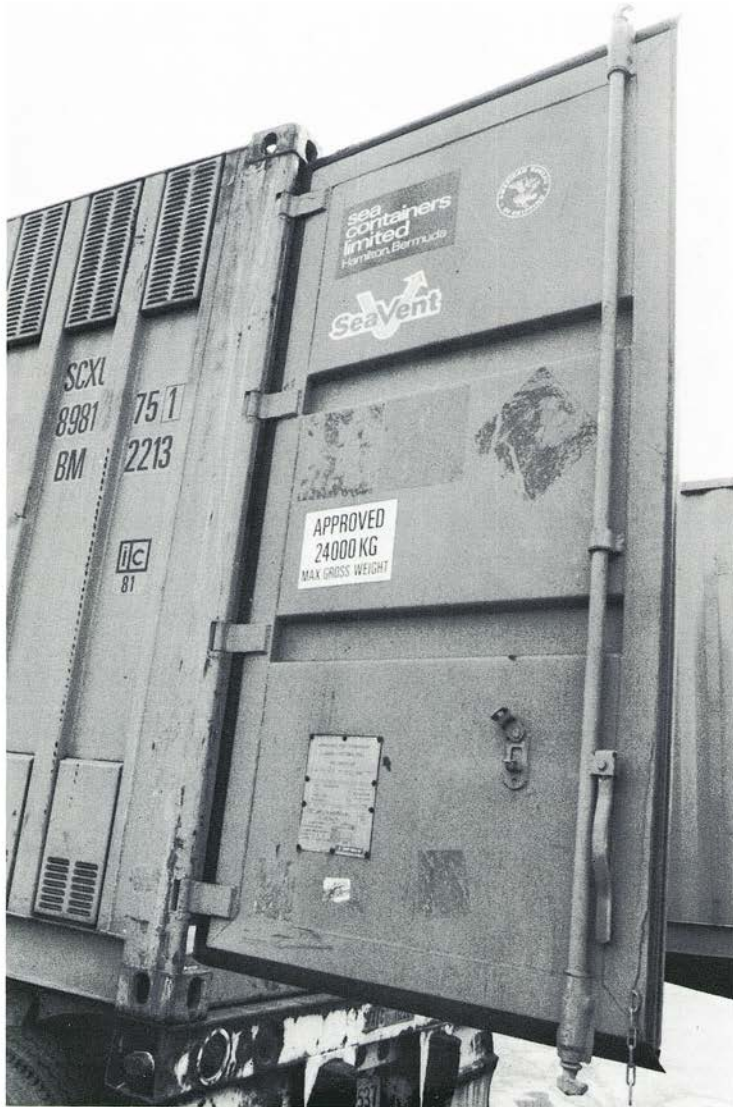
Fig. 1. Rear door of SCXU 898175-1. Note reverse corrugations on door.
