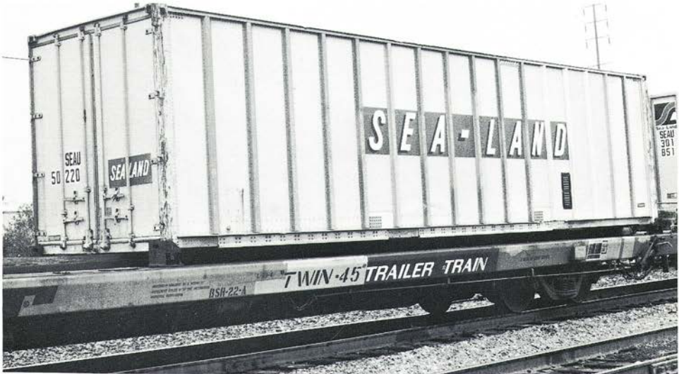
Fig.1. SEAU 50220. This entire series (SEAU 50000-series) of 35-foot dry van containers are off roster now. This container was built by Fruehauf. Note the number on the back (and front) only.
